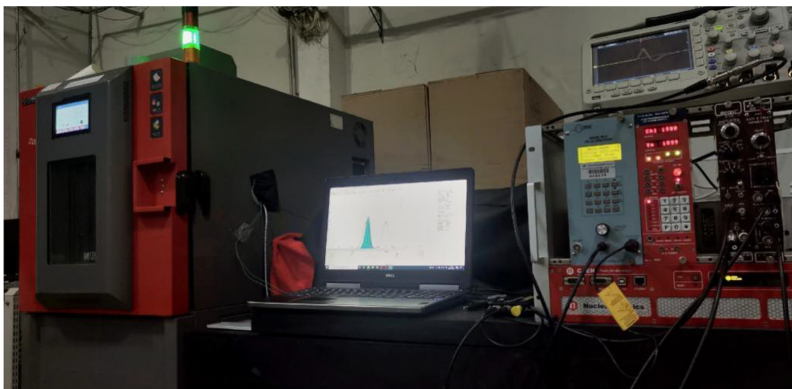
Fig. 8 Photograph of the experimental setup of temperature response of the HCC
