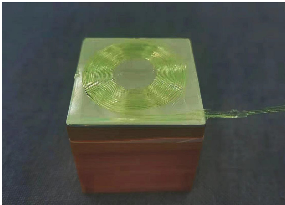
Fig. 1 The scheme of a HERD Calorimeter Cell. The crystal was wrapped with Enhanced Specular Reflector (ESR), and the above is WLSF pad, which is tightly attached to the crystal
